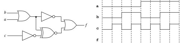
b) Complete the timing diagram of the logic circuit whose VHDL description is shown below: (7 pts)
